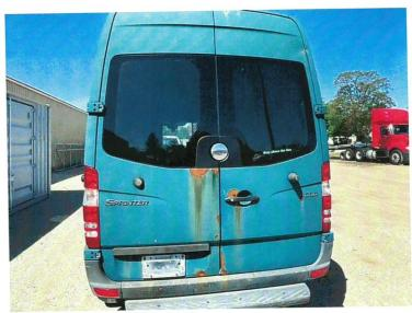
Van 24. Assigned to the maintenance technicians. This van has mechanical issues with the diesel emissions equipment. The Freightliner dealer quoted the department nearly \$6,000 to repair the problems. The van also has significant rust and paint issues. It is beyond economic repair. To be sent to auction.
