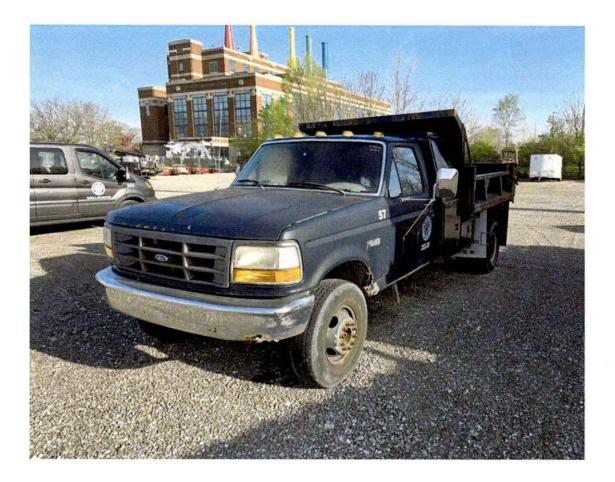
Truck 57. Originally assigned to grounds and then to landscape. This truck recently had an engine failure and was red tagged as unusable. It is a 28-year-old truck with expensive engine repairs required. The truck's value is less than the needed repairs. To be sent to auction.
